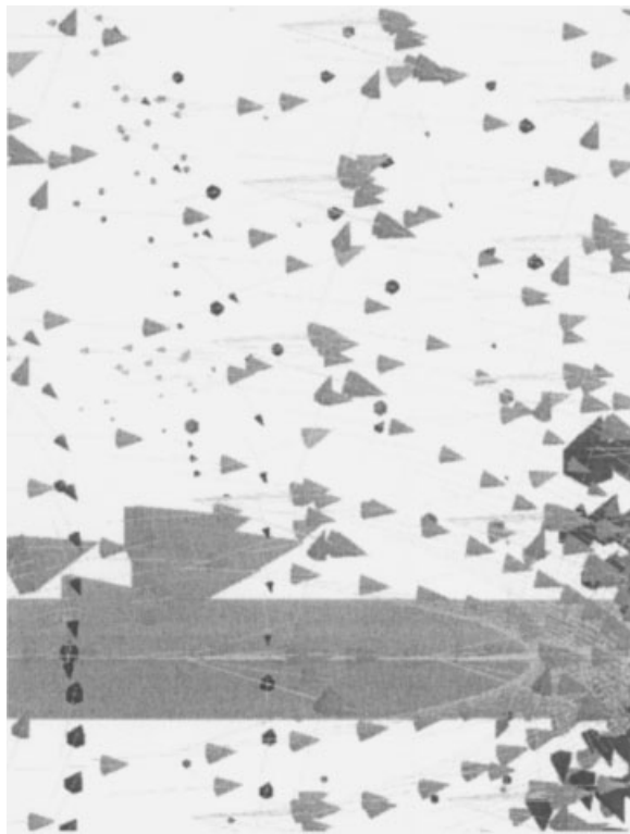
Figure 5. 3-D vectors indicating the presence of a leading-edge vortex.
